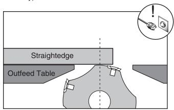
**Figure 46.** Adjusting outfeed table even with cutterhead body.
